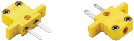
Type K ANSI illustrated (F37K-A). Recommended cutout: 8.5mm x 16.5mm
