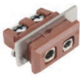
Recommended cutout: 13mm x 26mm. Type K illustrated (R34K)
