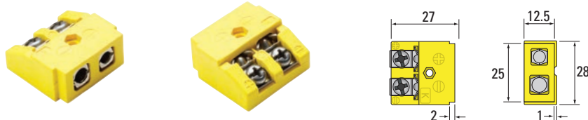
Type K ANSI illustrated (R28K-A) - see page 32 for mounting kit. Recommended cutout: 13mm x 25.8mm
