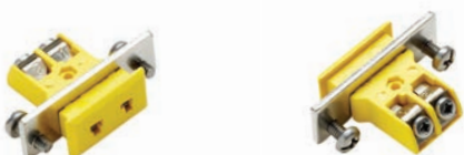
Type K ANSI illustrated (M29K-A). Recommended cutout: 6mm x 14mm
